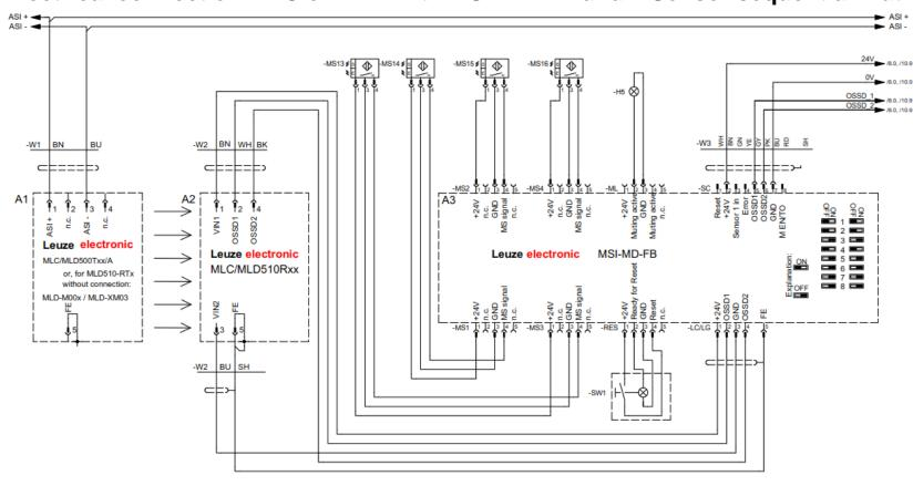
MSI-MD-FB + MLC510/MLD510 for ASI - coupling module sequence controlled 4-Sensor-Muting OM 54 Muting-timeout: 20sec
